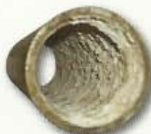
Galvanized Schedule 40 Pipe Untreated for 20 Months
